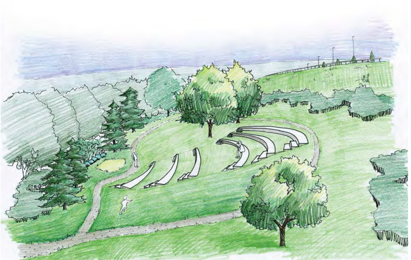
Sketch of proposed amphitheater. Pervious grass pavers are recommended for the stage area, providing a firm and level surface while also allowing for infiltration in storm events.
